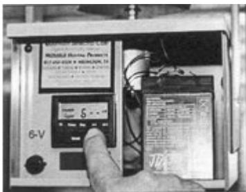
7 Press and release the timer button once. The timer should now say "TIMER 1, OFF". Press the hour (h+) key until 6 AM is shown.
