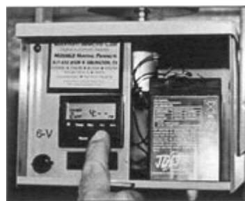
12 Press and release the timer button once. The timer should now say "TIMER 2, OFF". Press the hour (h+) key until 4 PM is shown.
