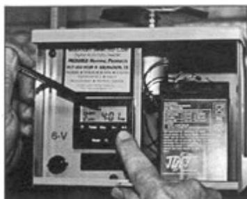
13 Press the minute (m+) key until :01 is shown. Remember that there should be all days showing in all feed times if you want the feeder to feed at those times all seven days a week.
