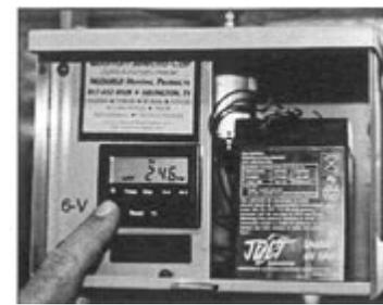
**Now test the unit and set the seconds of spin time.**
